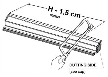
2 b: remove only the "handle bar" aluminum profile, which must be further cut by 6,8 cm (fixed size)
